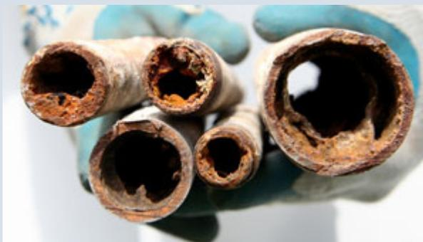
*Lead can attach to the corroded inside walls of a galvanized pipe if the water moves through a lead pipe before moving through the galvanized pipe. Lead can get into the water when pieces of the corrosion scale break loose, even after the lead service line is removed.*
