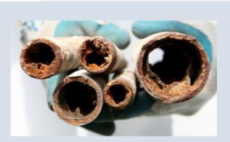
Lead can attach to the corroded inside walls of a galvanized pipe if the water moves through a lead pipe before moving through the galvanized pipe. Lead can get into the water when pieces of the corrosion scale break loose, even after the lead service line is removed.
