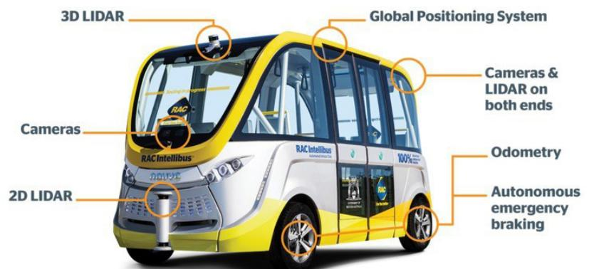
Figure 1.1 Navya sensor platform
