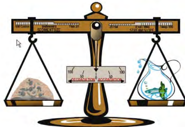
(Sediment LOAD) x (Sediment SIZE) ∝ (Stream SLOPE) x (Stream DISCHARGE) (Adapted from Lane, E. W., The Importance of Fluvial Geomorphology in Hydraulic Engineering , 1955)
