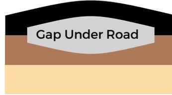
Water thaws, leaving voids under the pavement.
