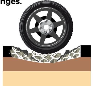
The weight of vehicles breaks the pavement which then collapses to form a pothole.
