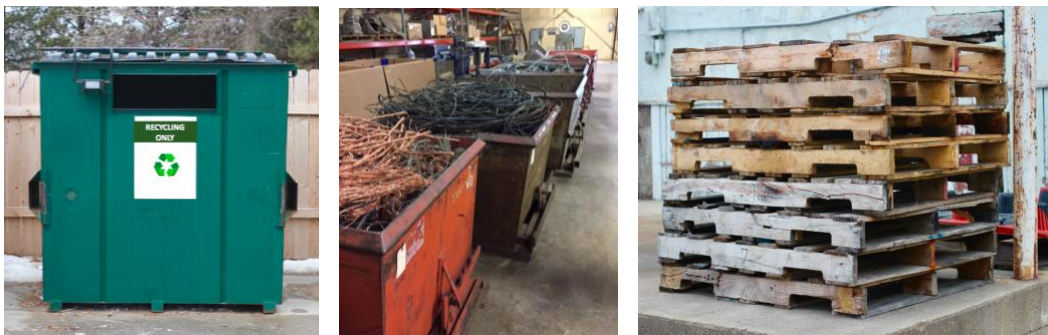
Recycling dumpsters with a cutout help reduce contamination (left). Scrap metal (center) and wooden pallets (right), among other things, can be collected and recycled (right).
