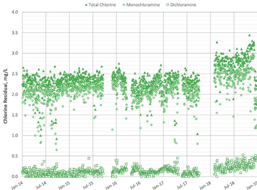
Figure 5-16 West Plant Finished Water Chloramine Speciation from January 2014 to January 2019
