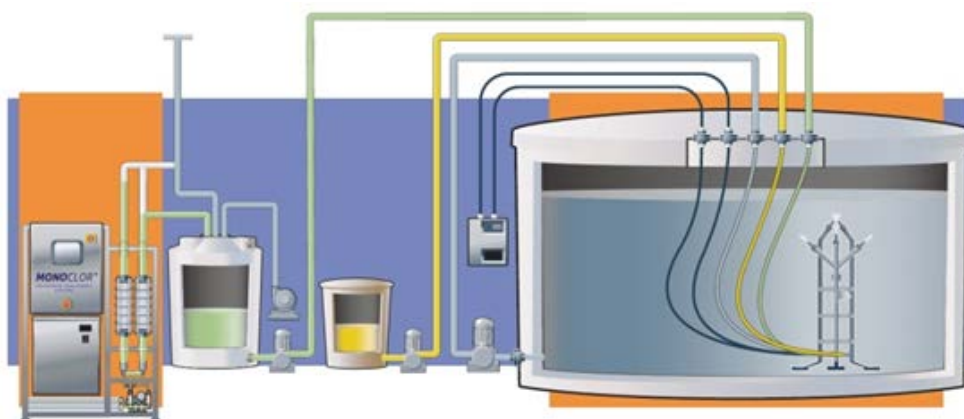
Figure 7-52 Process Schematic of UGSI Monochlor® Chloramine Booster System
