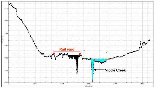
Figure 3-6 Modeled Cross Section with Blocked Obstruction
