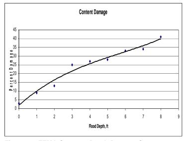
Figure 6-2 FEMA Contents Depth-Damage Curve
