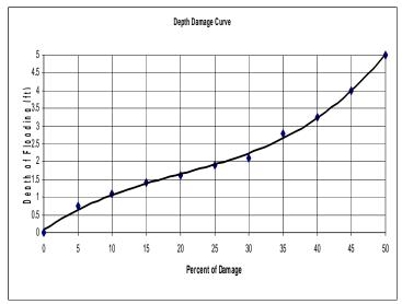
Figure 6-1 FEMA Building Depth-Damage Curve
