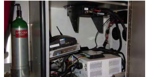
Crowded electronic compartment in an ambulance. WiFi, CDMA, GPS800, SMR—it's all in there
