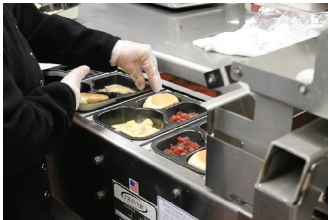
Meals are sealed using a specialized machine that keeps the foods from mixing during delivery.
