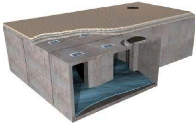
Parking lot subsurface storage detail
