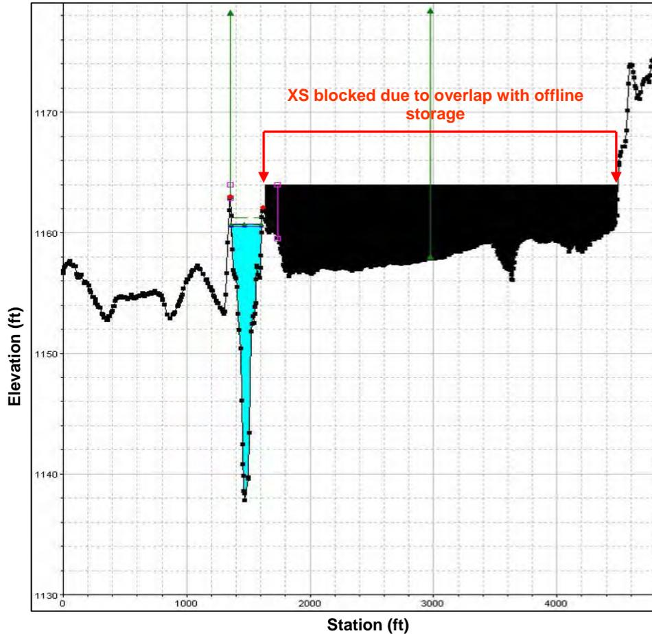
Figure 3-7 Cross Section of HEC RAS Blocked Obstruction
