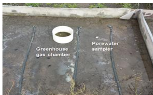
Fig. 7. Experimental plot set up with greenhouse gas chamber and pore-water sampler
