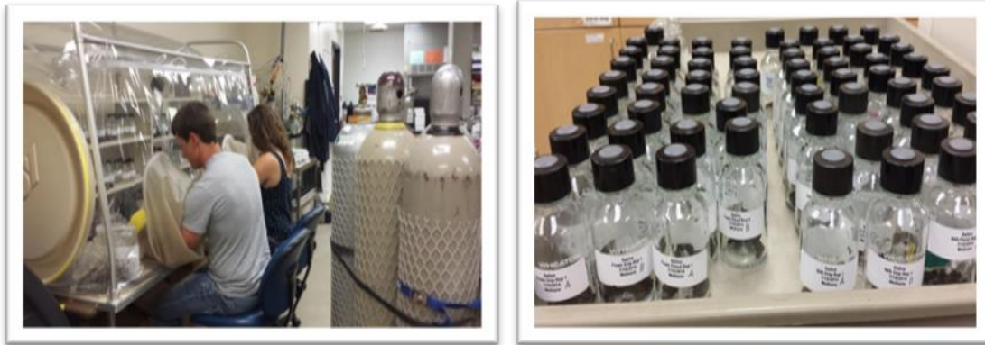
Fig. 8. Sediment core incubation experiment in the lab setting (Anaerobic glove bag and soil incubation for denitrification measurement)
