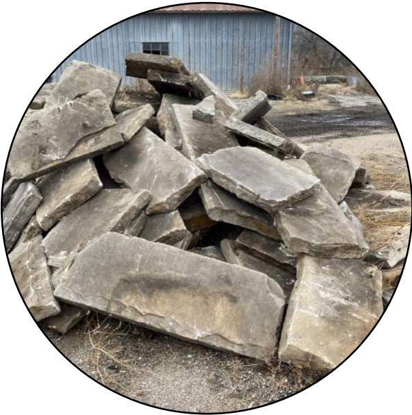
REUSED STONE CURBING FOR STORMWATER SEDIMENT FOREBAY
