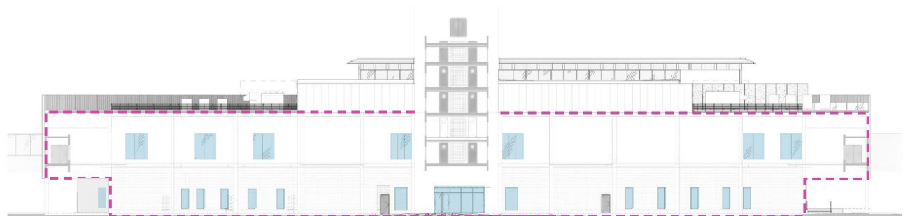
LEVEL 3 ADDITION WHITE PAINTED FACADE WINDOW OPENINGS FOR STAFF & PARTNER SPACES
