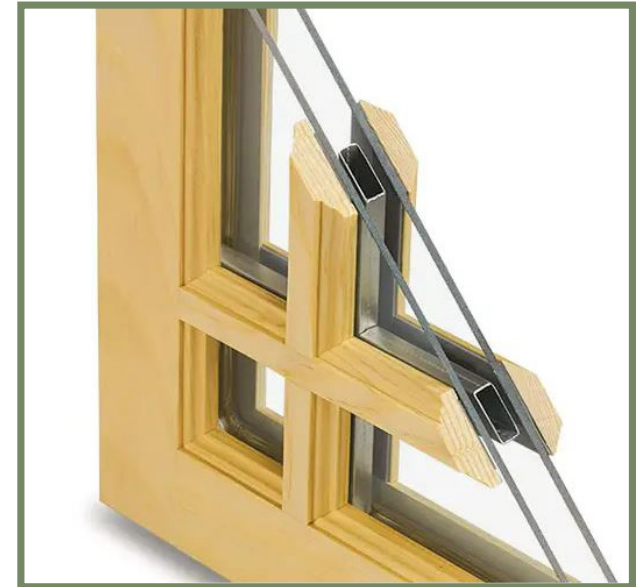
Simulated Divided Light with Spacer: two panes of glass are separated by a spacer bar with muntins applied on the outside of the glass.
