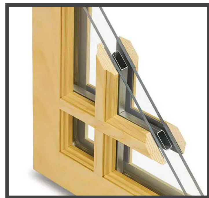
Simulated Divided Light with Spacer: two panes of glass are separated by a spacer bar with muntins applied on the outside of the glass.
