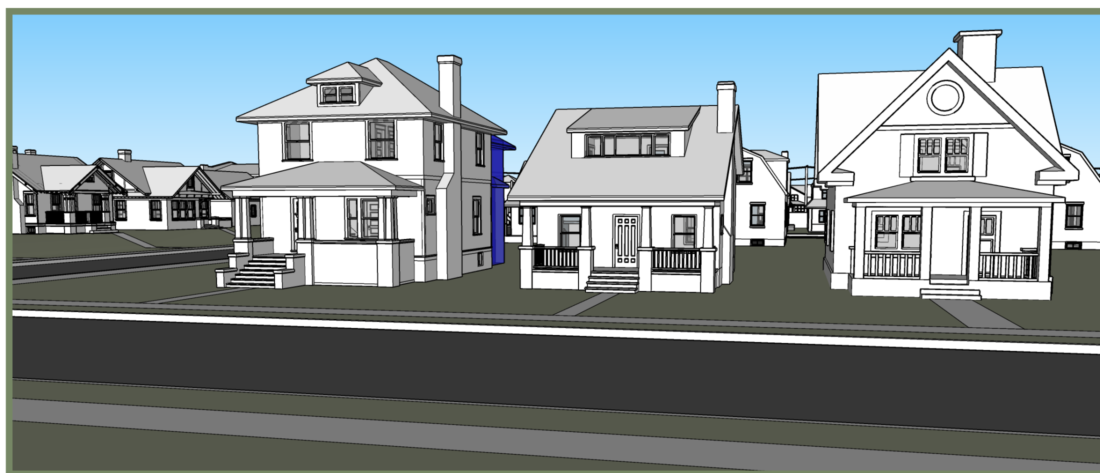
The minimum visual impact of the two story addition is created by inseting it from the side walls of the original home and scaling it down to be less than half the size of the original home.
