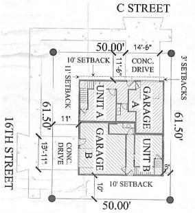
least five feet." Because the limited site area, garages are proposed to be in line with the main façade of the building. This does not meet the standard for garages.
