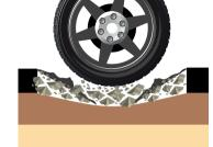
The weight of vehicles breaks the pavement which then collapses to form a pothole.
